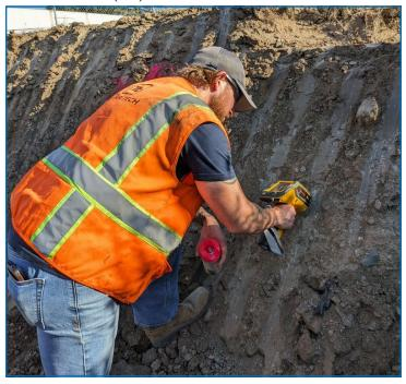
Air Force environmental contractor scans excavation sidewalls at CS 040 to determine soil composition by using an X-ray fluorescence (XRF) analyzer. XRF analyzers are one of the many tools environmental engineers and scientists are using in the cleanup effort at McClellan.
